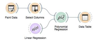
The Linear Regression widget provides two types of regularization. Ridge regression is the one we have talked about and minimizes the sum of squared coefficients  $\theta$ . Lasso regression minimizes the sum of absolute value of coefficients. Although the difference may seem negligible, the consequences are that lasso regression may result in a large proportion of coefficients  $\theta$  being zero, in this way performing feature subset selection.
