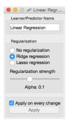
Here we go: we just reinvented regularization, a procedure that helps machine learning models not to overfit the training data. To observe the effects of the regularization, we can give Polynomial Regression our own learner, which supports these kind of settings.
