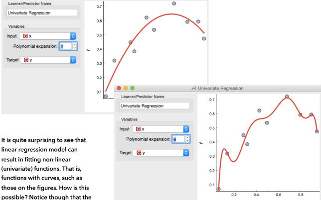
It is quite surprising to see that linear regression model can result in fitting non-linear (univariate) functions. That is, functions with curves, such as those on the figures. How is this possible? Notice though that the model is actually a hyperplane (a flat surface) in the space of many features (columns) that are powers of x. So for the degree 2,  $h(x)=\theta_0+\theta_1x+\theta_1x^2$  is a (flat) hyperplane. The visualization gets curvy only once we plot h(x) as a function of x.
