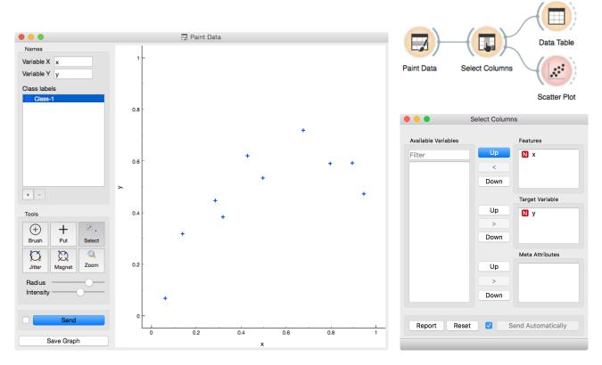
We would like to build a model that predicts the value of class y from the feature x. Say that we would like our model to be linear, to mathematically express it as  $h(x)=\theta_0+\theta_1x$ . Oh, this is the equation of a line. So we would like to draw a line through our data points. The  $\theta_0$  is then an intercept, and  $\theta_1$  is a slope. But there are many different lines we could draw. Which one is the best one? Which one is the one that fits our data the most?
